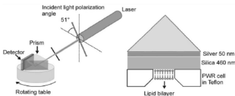
**Figure 1. PWR setup.** On the left the optical and mechanical components, the incident polarized light beam (a continuous wave He–Ne laser at 632.8 nm) is at 45° and the rotating table allows steps of 1 millidegree. On the right is a detailed view of the prism and the PWR cell sample with the lipid bilayer.
