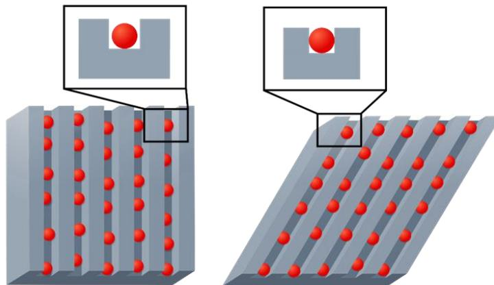
Figure: Schematic of the strain stiffening system with beads (red) inside the PDMS channels (grey). In the un-deformed state (left) the beads do not touch the channel walls. When the system is deformed the beads touch the walls.
